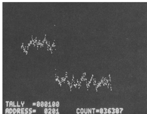
Fig. 5. Plot of light intensity at 250.5 nm vs. time after the flash in the photolysis of a mixture of \text{CH}_3\text{CHO} at 25.0 Torr and \text{O}_2 at 20.0 Torr at 310.5 nm. The time scale runs from left to right with a sweep time of 0.8 \mu\text{s} per channel. The fraction of light absorbed is 0.0043. The plot is an average of 100 shots.
